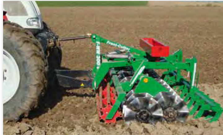
Front-Cutter WW „T“ with tube roller serves and front knife tine
